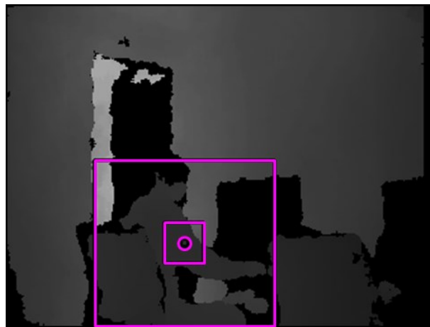
(b) Depth image of robot camera with human bounding box
