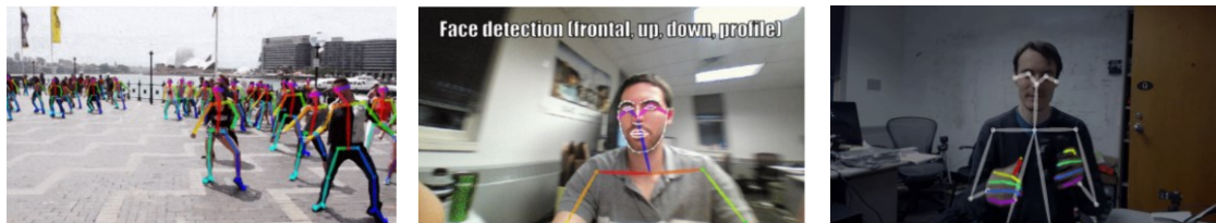
(a) Multiple people pose detection in RGB image (b) Face detection and upper limbs detections (c) A example of upper limbs and hands detection
